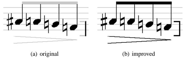
Fig. 3. Roach & Tatem’s original algorithm removes all horizontal shapes (marked grey), even when they do not lie on staff lines. This is resolved in our “improved” version.
