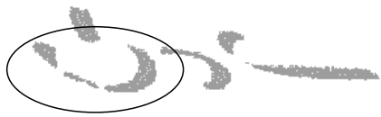
Figure 2: When the individual fragments of the marked broken symbol are classified, the estimator for the posterior probability might not be an appropriate confidence measure, because all class probabilities add to one, which ignores alternative segmentations. 1
